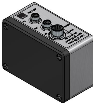
X0: Ethernet/IP IN: M8 4pin female
